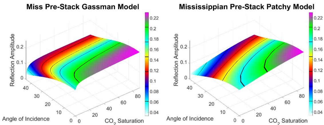
**Figure 1.** Pre-stack fluid substitution models of the Mississippian reservoir at Wellington Field. The plots show the modeled amplitude with respect to CO<sub>2</sub> saturation and angle of incidence. The black lines are amplitude contours.
