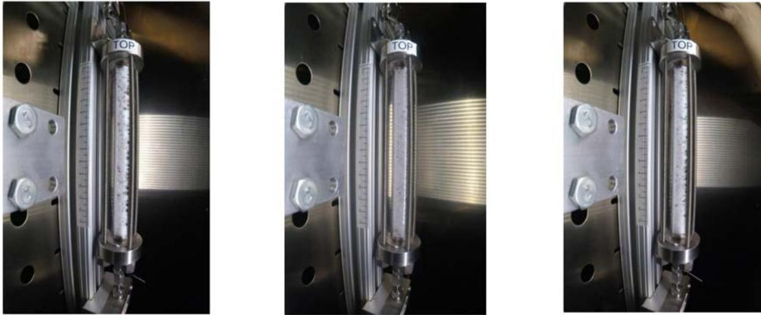
**Figure 1.** Foams generated without crude oil with surfactant (left) surfactant-PEI (middle) and surfactant-NP (right) at 40 °C and 1300 psi.
