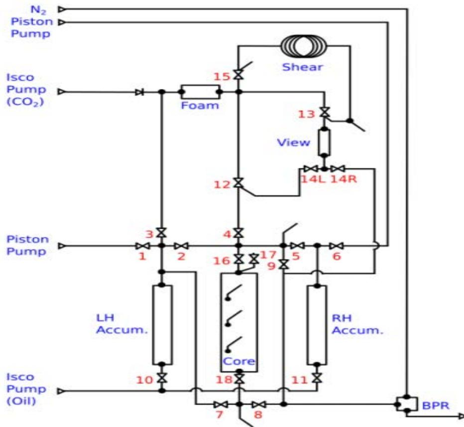
**Figure 2.** Core flood system prepared for the injection of CO<sub>2</sub>-foam into a long core either 100% saturated with brine or brine at residual oil saturation.
